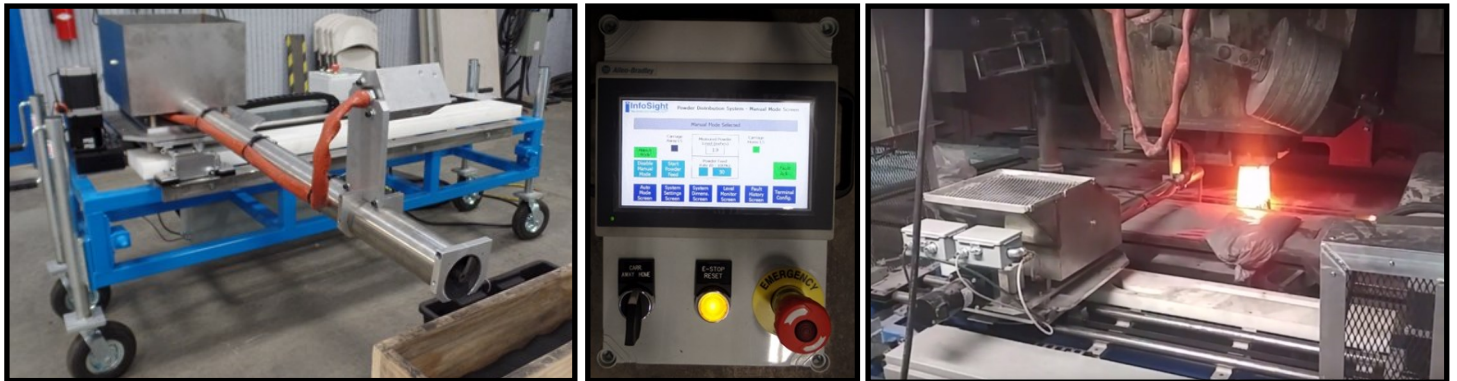
Left: The Mold Powder Feeder at the InfoSight shop. Middle: The Control Panel. Right: The Mold Powder Feeder in Action at a steel mill.
